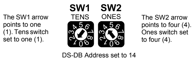
Figure 2.27 DS-DB Address Switches
